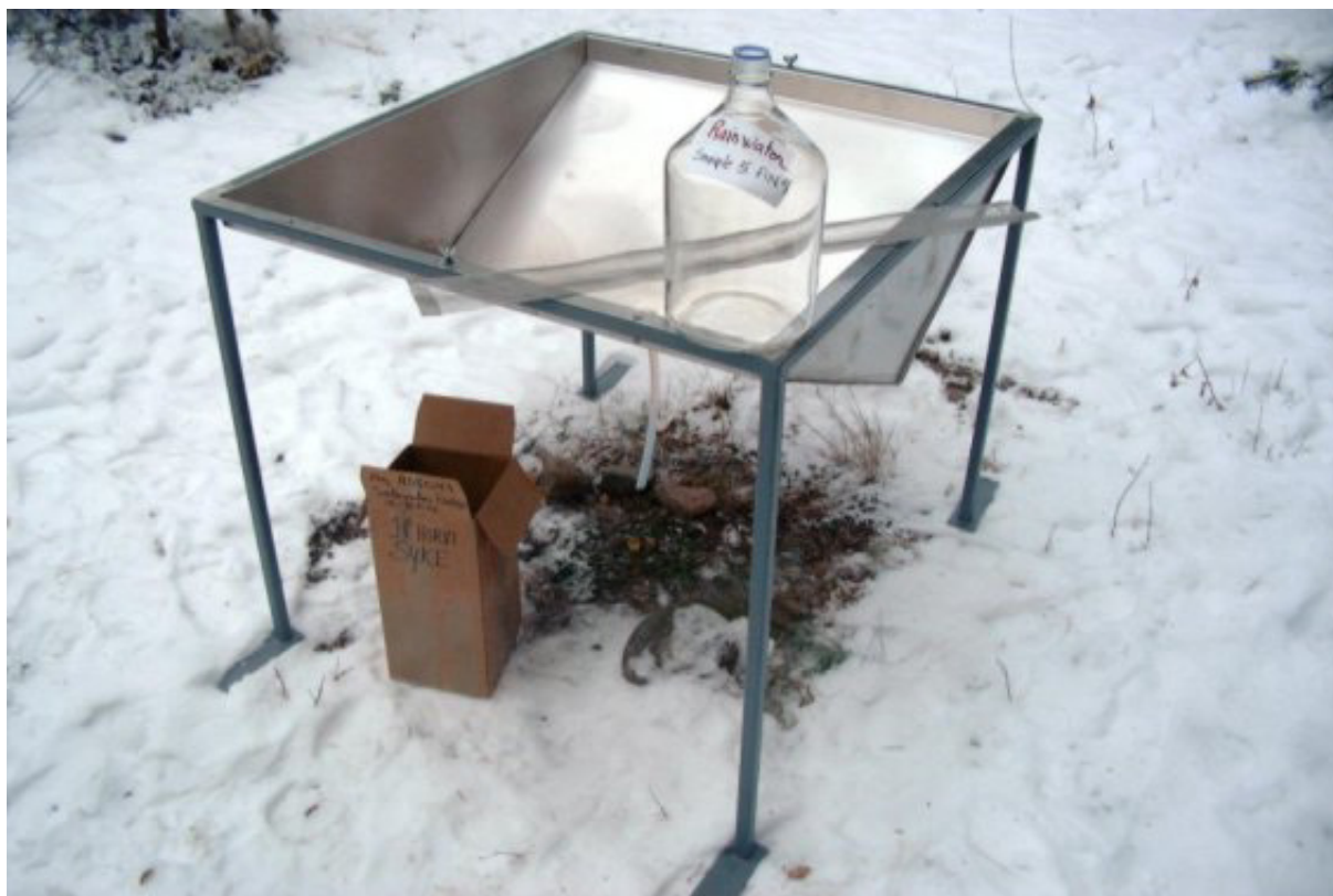
FIGURE 3. Pieces and tools for sampling of rain water in Southern Finland. Photo taken 14 th November 2002. Joint Nordic screening project on musk substances. Finnish Environment Institute (SYKE).
